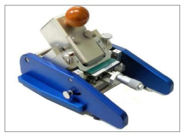
This new accessory is very unique and convenient tool to cut the samples in several micron thickness. Angle can be set at any angle between 45 degree to 90 degree. Because of its unique mechanics, it can be used for not only soft samples like films but also hard samples like plastic.
